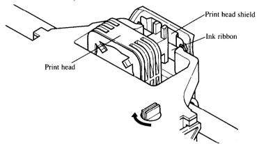
3 Use the grips on the side of the ribbon cartridge to help locate the cartridge (squeeze them inwards gently), and make sure that the spindles on the cartridge holder fit into the sockets on the cartridge itself.
