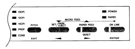
The principle involved is that the printer will print a list of options on one line. You use the set/DEET and page buttons to move the print head so that it is below the option you want to choose.
